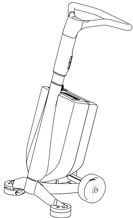
Fig. 17 GuardianWeld induction machine Welds the GWSP(*)-80-F2E/F4E to PVC, TPO and EPDM membranes
