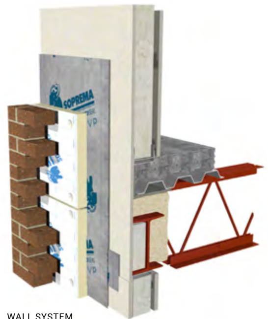
WALL SYSTEM BUILDUP
