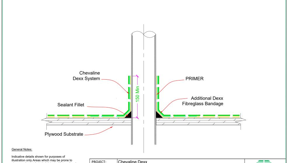
Indicative details shown for purposes of illustration only. Areas which may be prone to stress such as substrate joints, and internal and external corners are to be treated with a double layer of fibreglass mat. This drawing is to be read in conjunction with the New Zealand building code, and NZS 3604 to determine structural framing and deck substrate dimensions, materials, and treatment, and also minimum falls
