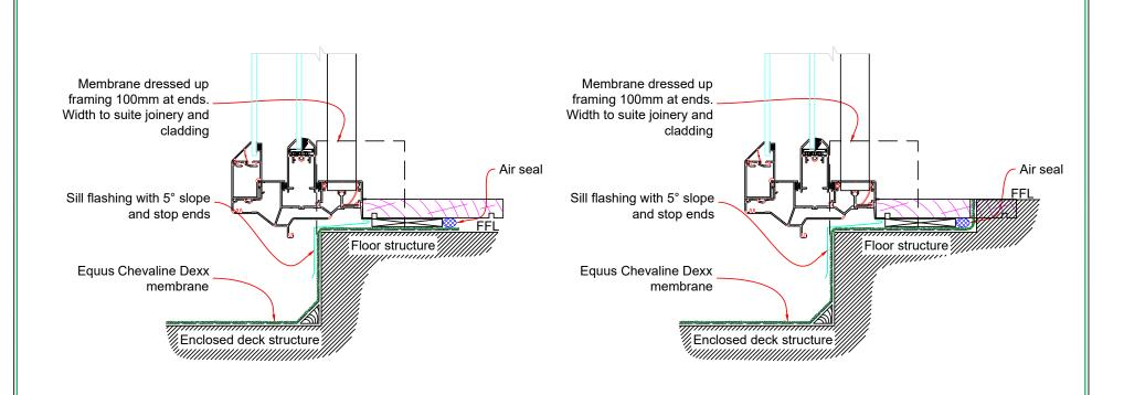
Indicative details shown for purposes of illustration only. Areas which may be prone to stress such as substrate joints, and internal and external corners are to be treated with a double layer of fibreglass mat. This drawing is to be read in conjunction with the New Zealand building code, and NZS 3604 to determine structural framing and substrate dimensions, materials, and treatment, and also minimum step down between floor and deck levels.
