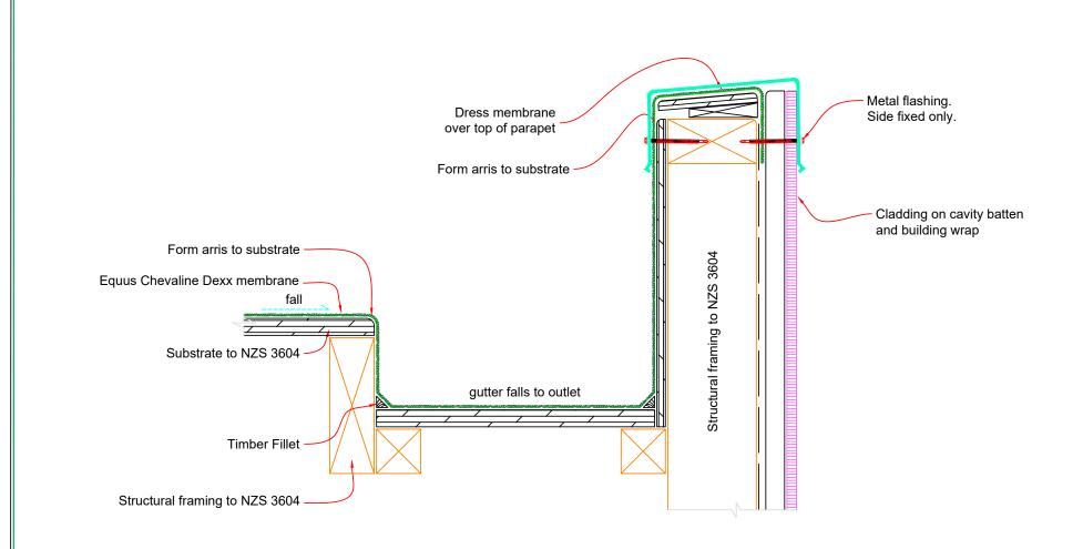
Indicative details shown for purposes of illustration only. Areas which may be prone to stress such as substrate joints, and internal and external corners are to be treated with a double layer of fibreglass mat. This drawing is to be read in conjunction with the New Zealand building code, and NZS 3604 to determine structural framing and deck substrate dimensions, materials, and treatment, and also minimum falls, overlapping, and minimum gutter dimensions.
