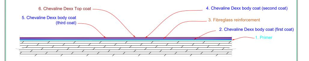
Indicative details shown for purposes of illustration only. Areas which may be prone to stress such as substrate joints, and internal and external corners are to be treated with a double layer of fibreglass mat. This drawing is to be read in conjunction with the New Zealand building code, and NZS 3604 to determine structural framing and deck substrate dimensions, materials, and treatment, and also minimum falls, overlapping and outlet size.
