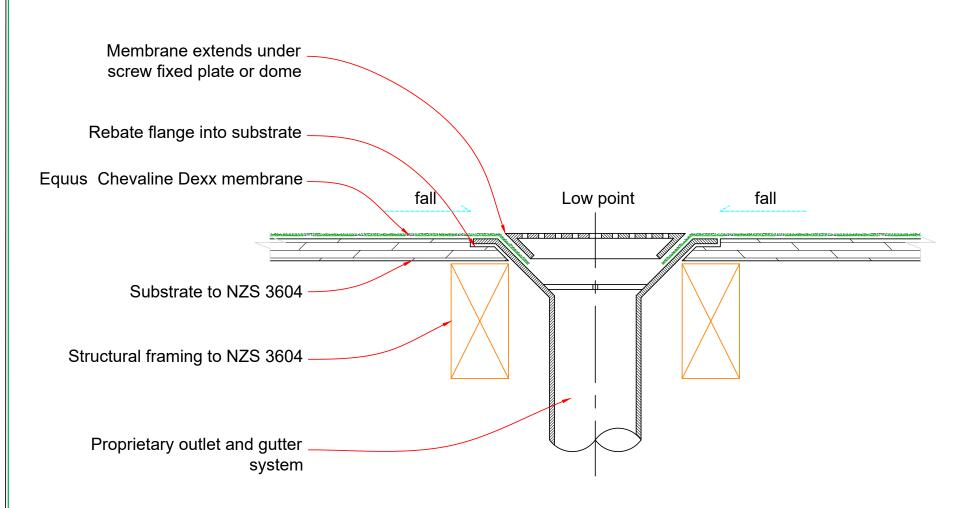
Indicative details shown for purposes of illustration only. Areas which may be prone to stress such as substrate joints, and internal and external corners are to be treated with a double layer of fibreglass mat. This drawing is to be read in conjunction with the New Zealand building code, and NZS 3604 to determine structural framing and deck substrate dimensions, materials, and treatment, and also minimum falls
