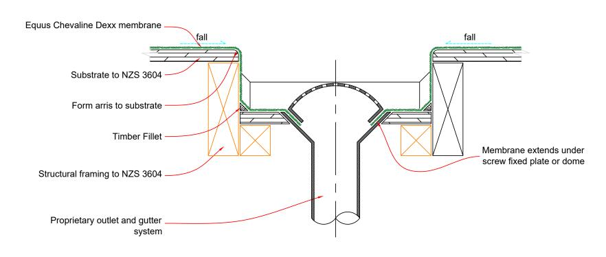
Indicative details shown for purposes of illustration only. Areas which may be prone to stress such as substrate joints, and internal and external corners are to be treated with a double layer of fibreglass mat. This drawing is to be read in conjunction with the New Zealand building code, and NZS 3604 to determine structural framing and deck substrate dimensions, materials, and treatment, and also minimum falls, overlapping, and minimum gutter dimensions.
