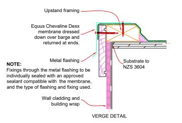
Indicative details shown for purposes of illustration only. Areas which may be prone to stress such as substrate joints, and internal and external corners are to be treated with a double layer of fibreglass mat. This drawing is to be read in conjunction with the New Zealand building code, and NZS 3604 to determine structural framing and substrate dimensions, materials, and treatment, and also minimum falls, overlapping and spouting size.
