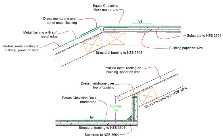
Indicative details shown for purposes of illustration only. Areas which may be prone to stress such as substrate joints, and internal and external corners are to be treated with a double layer of fibreglass mat. This drawing is to be read in conjunction with the New Zealand building code, and NZS 3604 to determine structural framing and substrate dimensions, materials, and treatment, and also minimum falls.
