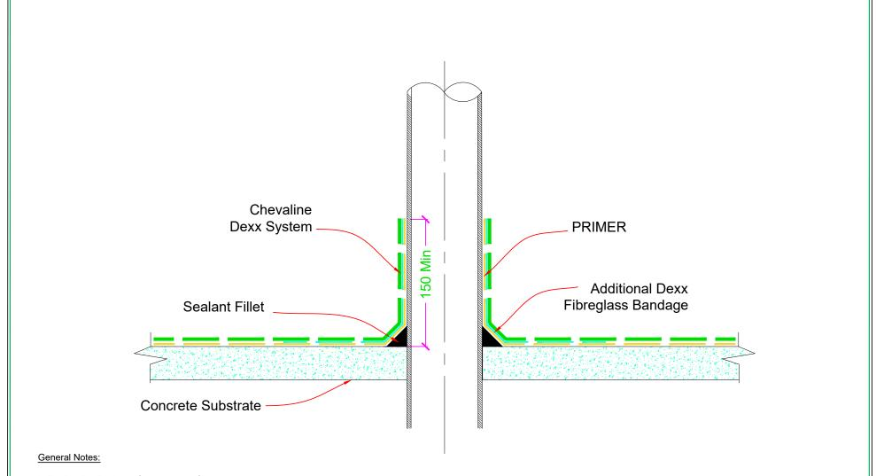
Indicative details shown for purposes of illustration only. Areas which may be prone to stress such as substrate joints, and internal and external corners are to be treated with a double layer of fibreglass mat. This drawing is to be read in conjunction with the New Zealand building code, and NZS 3604 to determine structural framing and deck substrate dimensions, materials, and treatment, and also minimum falls
