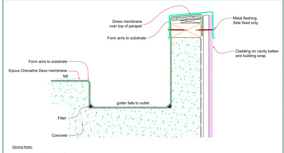
Indicative details shown for purposes of illustration only. Areas which may be prone to stress such as substrate joints, and internal and external corners are to be treated with a double layer of fibreglass mat. This drawing is to be read in conjunction with the New Zealand building code, and NZS 3604 to determine structural framing and deck substrate dimensions, materials, and treatment, and also minimum falls, overlapping, and minimum gutter dimensions.
