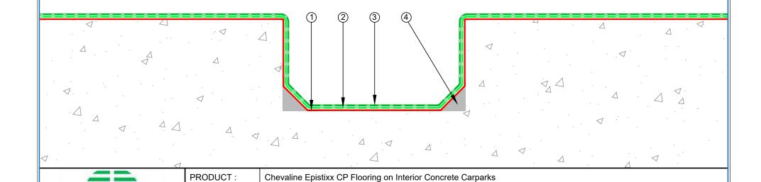
Standard channel drain detail
