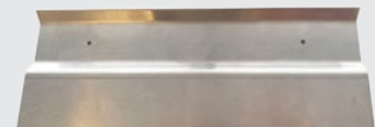
TERMINATION BAR A pre-manufactured profile that terminates the waterproofing membrane at the wall in a professional and watertight, wind-peel resistant manner with the addition of 50 mm flange for securing drainage board.
